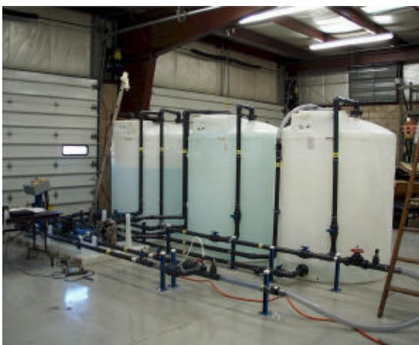
**Fig. 14: Multiphase flow loop for testing sensors. From left to right, tanks are for mineral oil, water and collection (mixture).**
